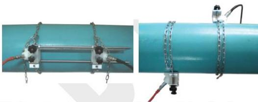
**M-Mounting Frame (V method and Z method)**
