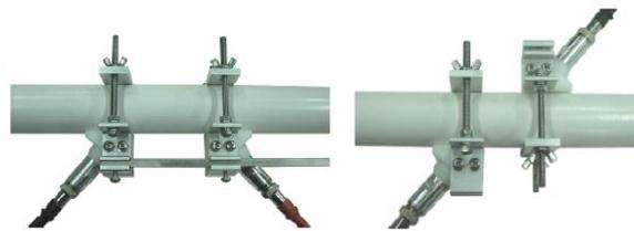
**S-Mounting Frame (V method and Z method)**
